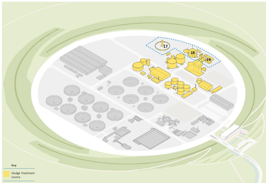
Figure 2.15: Flare (17), gas bag (18) and biogas upgrading plant (19) location
